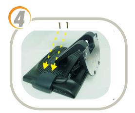
Align and insert mounting screws into holes and tighten using a Philips screwdriver.
