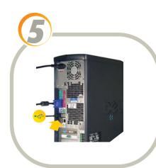
Attach USB cable from MSR device to the USB port on the rear of the computer.
